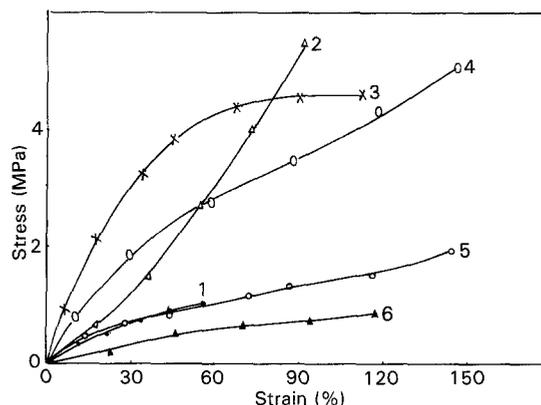
Figure 7 Stress-strain curves of System A<sub>3</sub> at different temperatures (°C): (1) 10; (2) 20; (3) 28; (4) 50; (5) 70; (6) 100.
