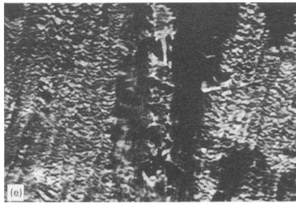
Figure 2 SE micrographs showing the surface morphology of fractured Ca-g-AN film at different temperatures (°C): (a) 28 (60 ×); (b) 40 (60 ×); (c) 80 (150 ×); (d) 100 (150 ×); (e) magnified view of (350 ×).
