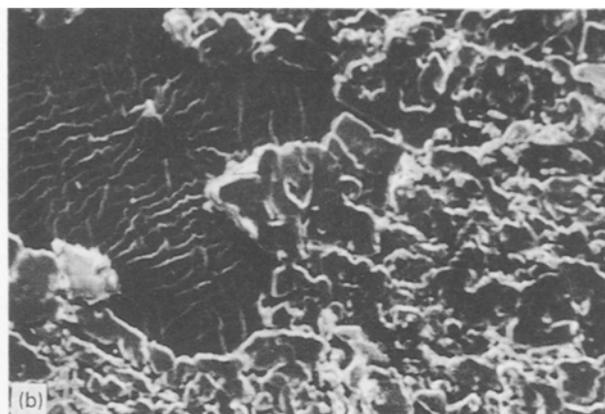
Figure 5 SE micrographs showing the surface morphology of 10% strained Ca-g-AN-co-nBMA films (System A). (a) A<sub>1</sub> (650 ×); (b) A<sub>3</sub> (650 ×).
