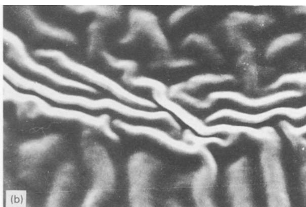
Figure 6 SE micrographs showing the surface morphology of System B<sub>3</sub>. (a) Unstretched (900 ×); (b) magnified view of (4500 ×).
