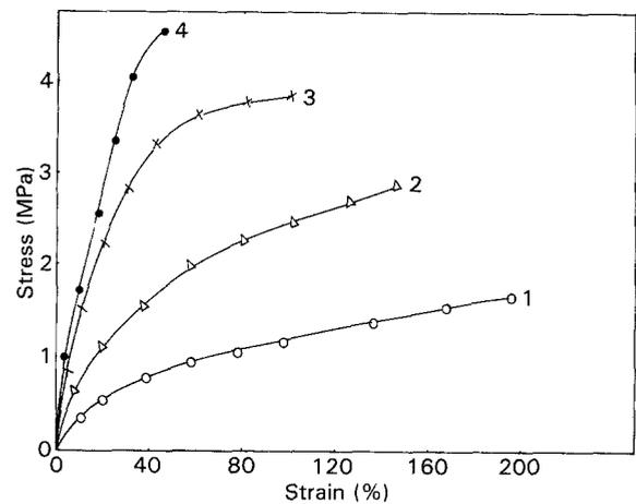
Figure 4 Stress-strain behaviour of System B (0.8:0.2). 1 = 0.4 mol dm<sup>-3</sup>; 2 = 0.8 mol dm<sup>-3</sup>; 3 = 1.2 mol dm<sup>-3</sup>; 4 = 1.6 mol dm<sup>-3</sup>.
