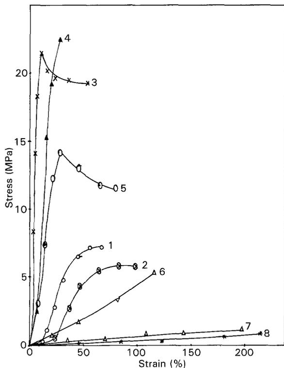
Figure 1 Stress-strain curves of Ca-g-AN at different temperatures ( $^{\circ}\text{C}$ ).
