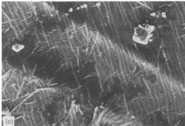
Figure 9 SE micrographs showing the fractured surface of System A<sub>3</sub> tested at different temperatures (°C) (600 ×): (a) 50; (b) 70; (c) 100.
