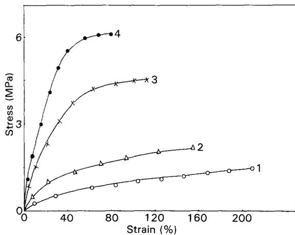
Figure 3 Stress-strain behaviour of System A (0.9:0.1). 1 = 0.4 mol dm<sup>-3</sup>; 2 = 0.8 mol dm<sup>-3</sup>; 3 = 1.2 mol dm<sup>-3</sup>; 4 = 1.6 mol dm<sup>-3</sup>.
